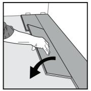
[6] Second plank, second row. Place the board tight to the short end of the previous panel. Insert the long end (tongue) into the first rows long end (groove). Insert at an angle then fold down in a single action movement.
