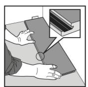
[2] Second plank, first row. Place next floor board tight to the short end of the first plank in the
