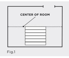
• Do a dry layout of the planks from the chalk line to check the widths of the end rows. These border rows should not be less than half of the plank width. If they are, move the starting line so that the room would be in balance and allow for larger cut piece at the ends.
