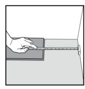
[4] At the end of the first row, measure the length of the last plank, making sure to leave a 10mm expansion gap.
