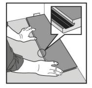
[2] Second plank, first row. Place next floor board tight to the short end of the first plank in the corner
