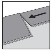
[1] First plank, first row. Start in the left hand corner of the room with the locking strip (groove) facing the room.
