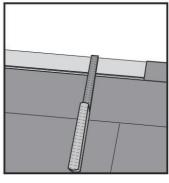
[8] Last row (and perhaps first row). Minimum floor board width 35mm. Remember to leave expansion gap of 12–15mm.
