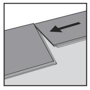
[1] First plank, first row. Start in the left hand corner of the room with the locking strip (groove) facing the room. Remember to leave a 12-15mm expansion gap between the wall(left) and the board. It is more practical to adjust the expansion gap between the long side and the wall.
